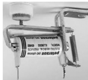
Illustration 2: Peterson version of chest magnet. Note the more robust coil spring.
